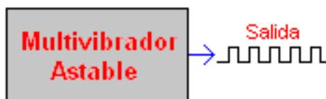
*Figura 9: Multivibrador Astable*
