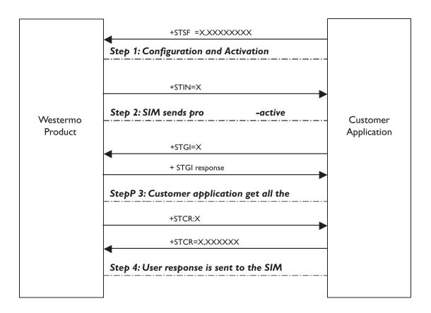
On the first step, the customer application informs the WESTERMO product which facilities are supported. This operation is performed with the +STSF (SIM ToolKit Set Facilities) command, which also allows to activate or deactivate the SIM Toolkit functionality.
