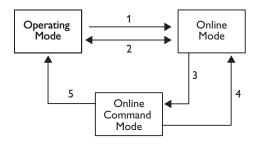
Example of commands/events that can trigger a change of the modems operation modes
