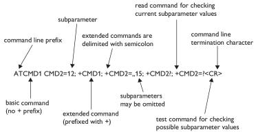
Figure 1: Basic structure of a command line
